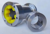
•This non- lubricated coupling accommodates for misalignment without loss of performance. The ease of high quality polyurethane insert replacement significantly reduces maintenance cost and minimal downtime while safeguarding your employees and equipment. This coupling is suitable for moderate to high speed operation on a wide range of general purpose motors and turbine driven equipment.
